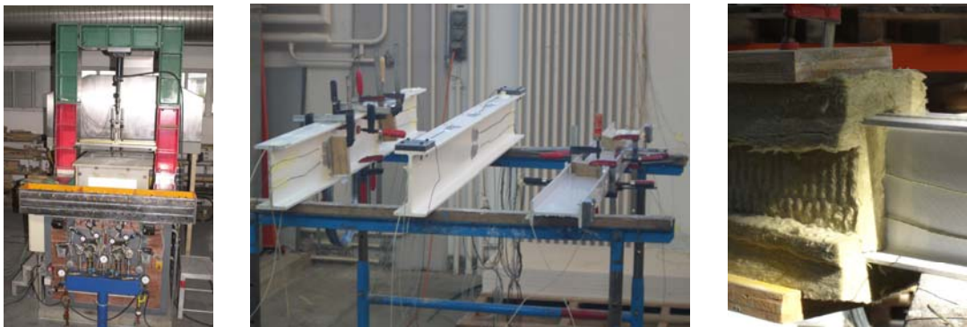
Figure 4. Small furnace with test setup, application of measuring points at the different profile types and a 50 mm mineral wool protected IPE 120
