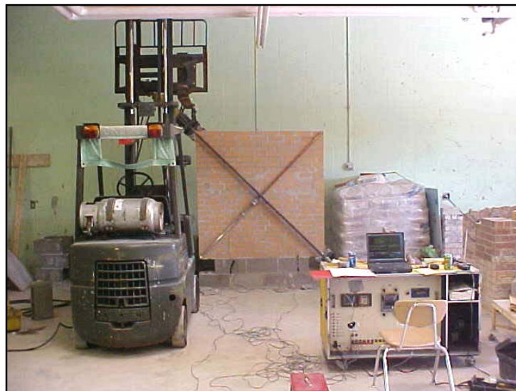
Fig. 3.4b Test setup for clay panel
