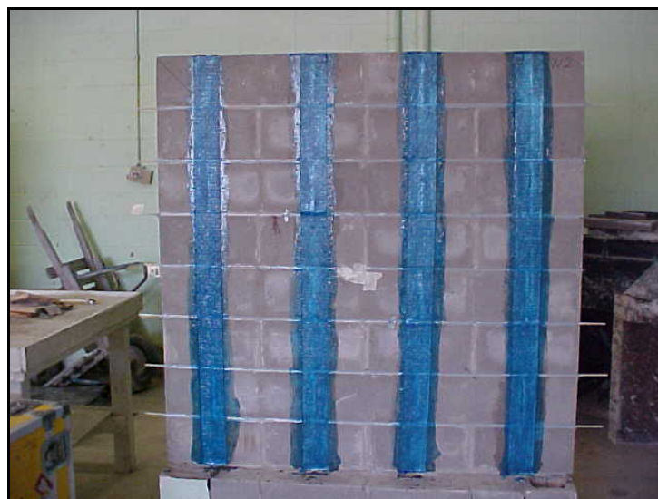
Fig. 3.3.4o Strengthened panel with GFRP laminates and rods
