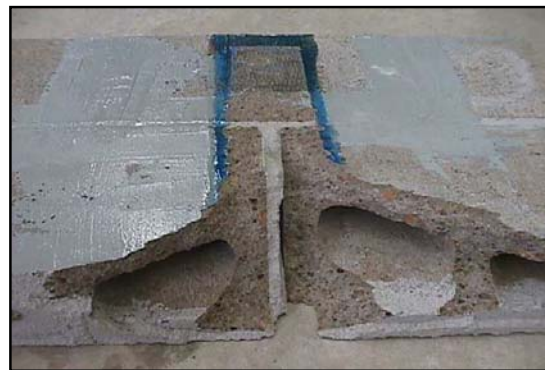
Fig. 2.3.5c 45° Fractures on the second course of concrete units
