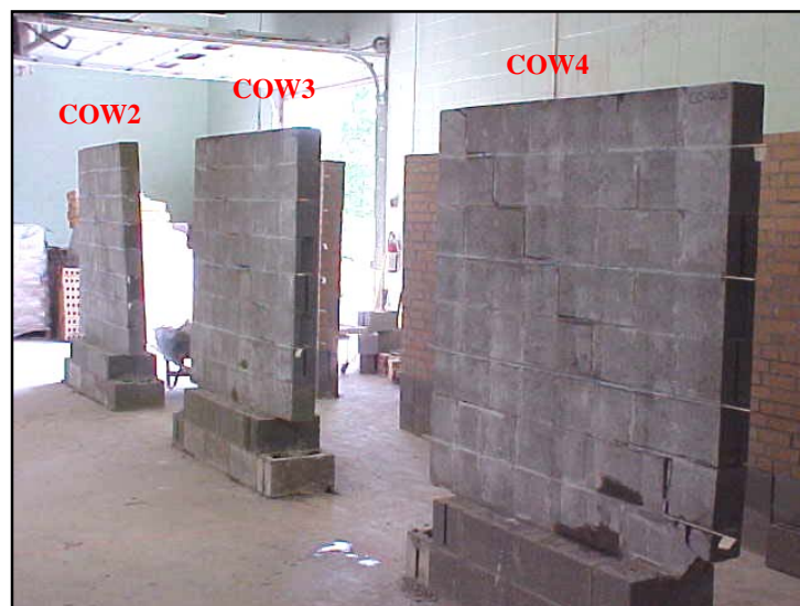
Fig. 3.5.3.1c Strengthened specimens after collapse
