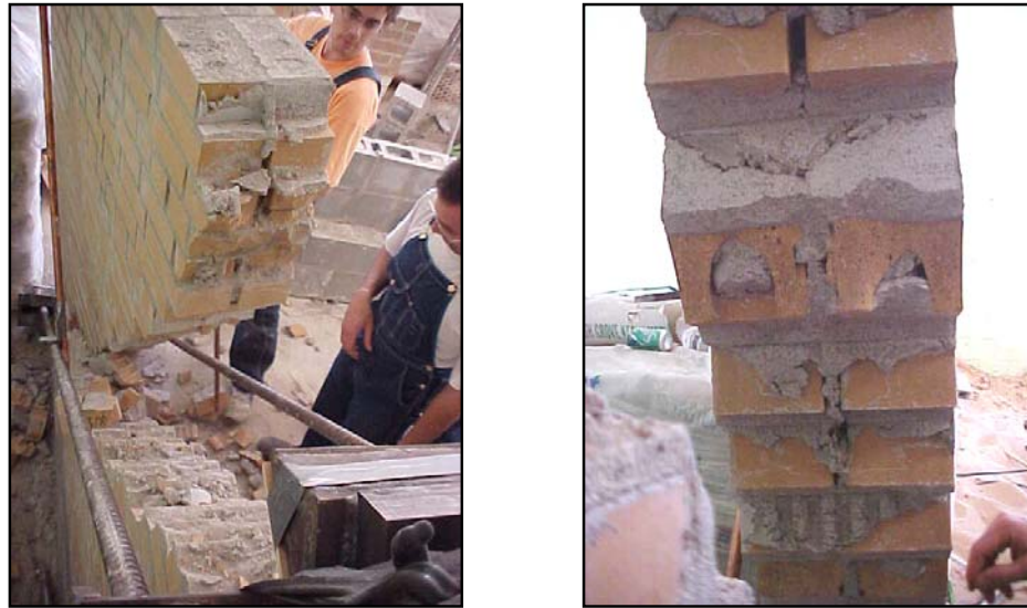
Fig. 3.5.3.2a(left)-b(right) Splitting of clay units in CLW1
