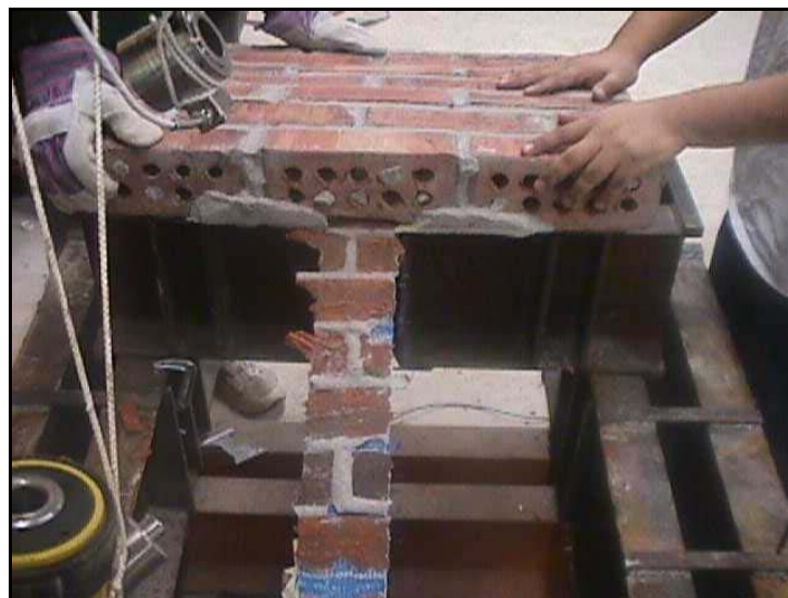
Fig. 2.3.5b** Debonded FRP laminate after failure
