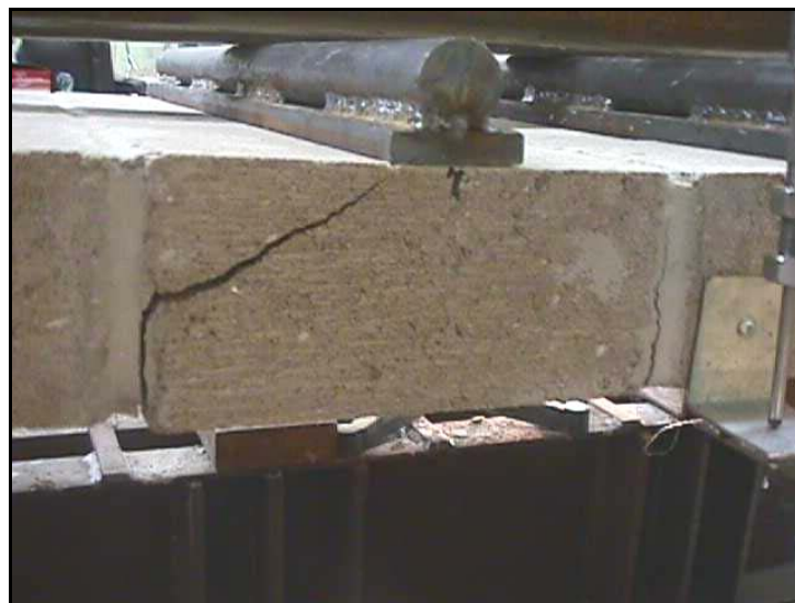
Fig. 2.3.5f Developing of flexural-shear crack under a loading point
