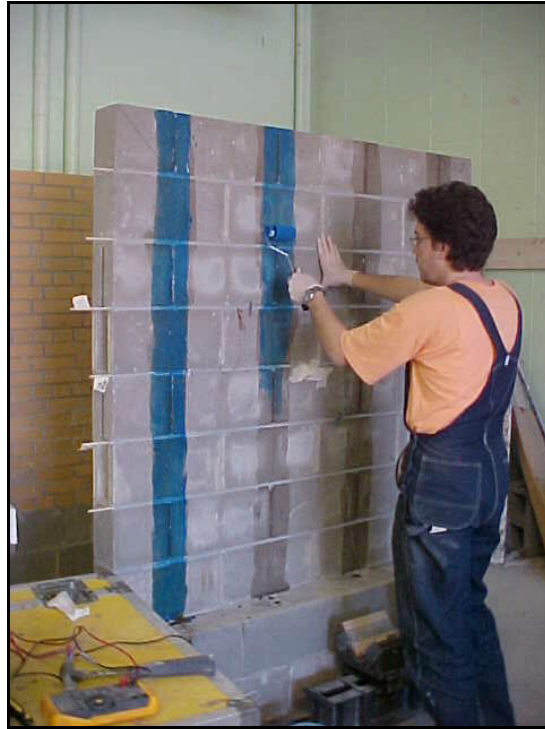
Fig. 3.3.4l 1 st coat of saturant
