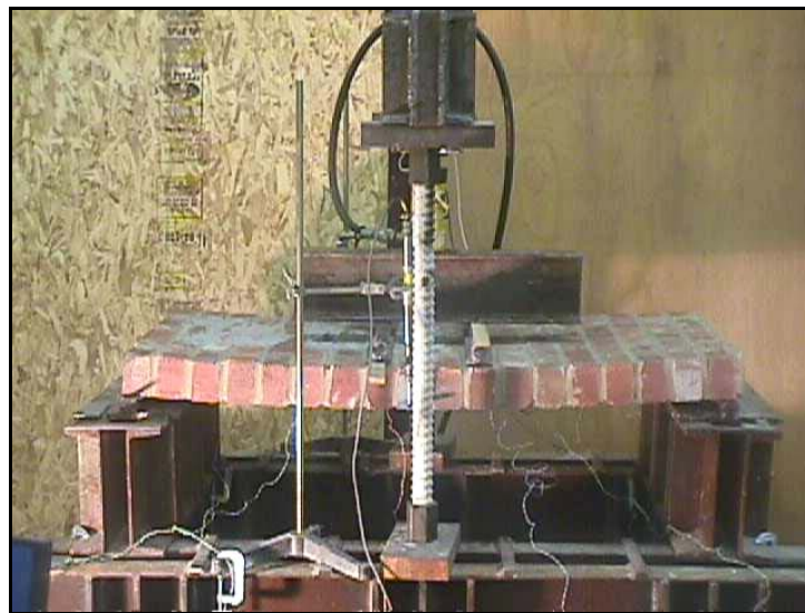
Fig. 2.3.5j** Wall deflection at the ultimate stage
