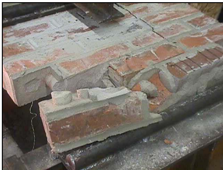
Fig. 2.3.51** Slipping in the vertical direction of the first mortar joint
