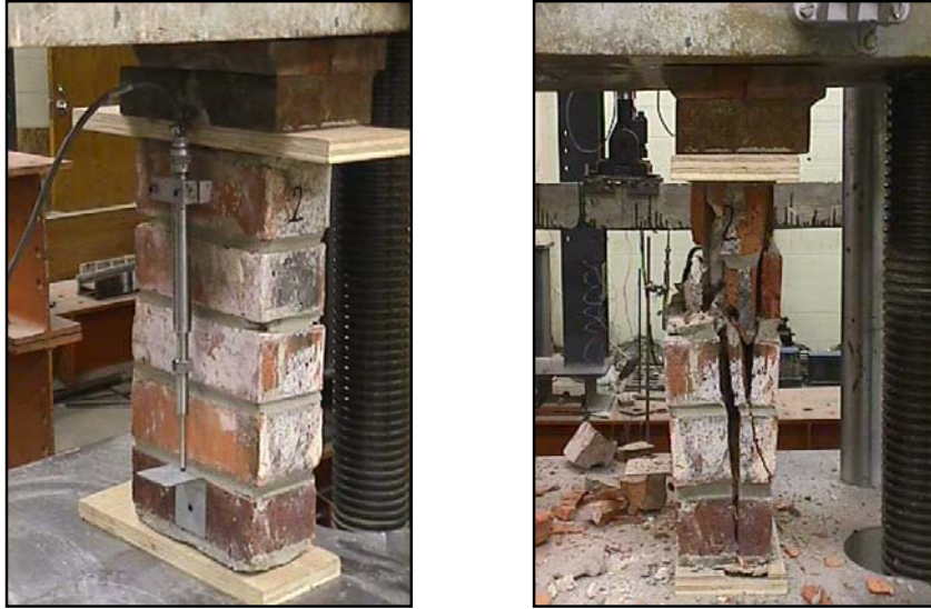
Fig. A.2.1b-c Dark clay prism before (left) and after failure (right)
