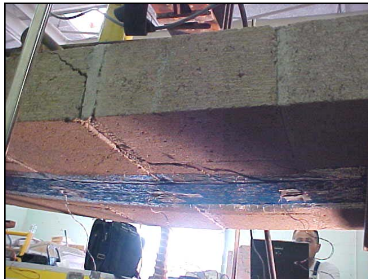
Fig. 2.3.5h Flexural-shear behavior at the final stage
