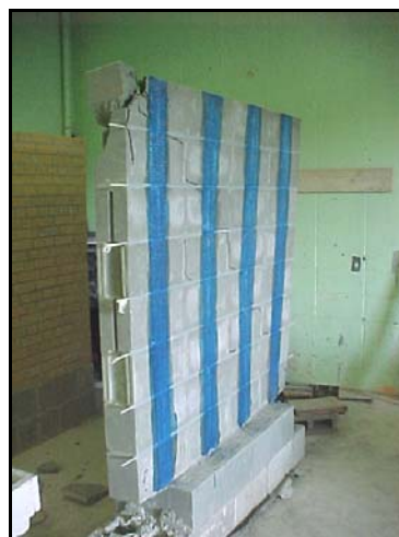
Fig. 3.5.1l Strengthened side of the panel after collapse
