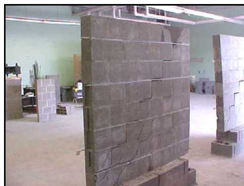
Fig. 3.5.1f Panel after failure
