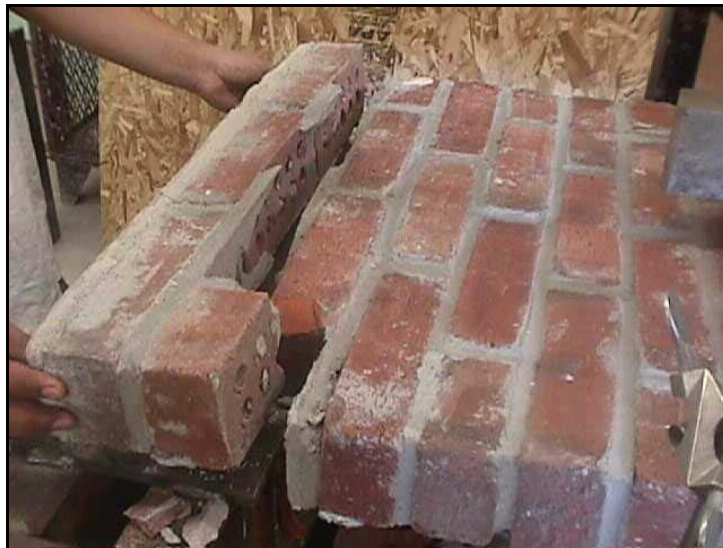
Fig. 2.3.5n** Slipping of the mortar joint at the border
