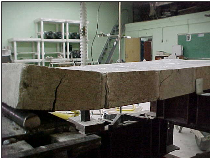
Fig. 2.3.5j* Developing of shear cracks for the entire length
