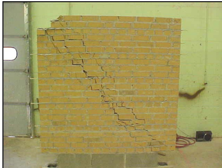
Fig. 3.5.2h Crack pattern of CLW4
