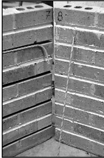
Fig. 3.2d GFRP rods in mortar bed joints (Tinazzi)
