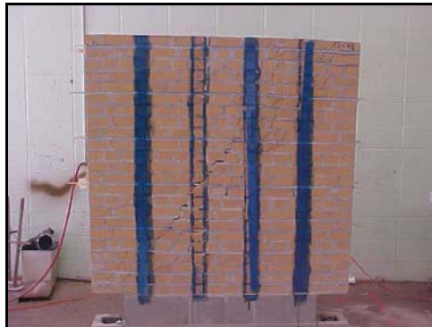
Fig. 3.5.2f Panel after failure
