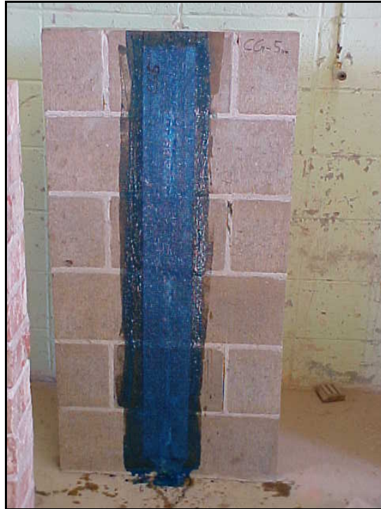
Fig. 2.3.3j Reinforced specimen before testing
