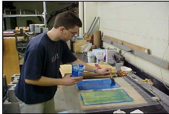
Fig. A.4.4a Final impregnation of laminate plies
