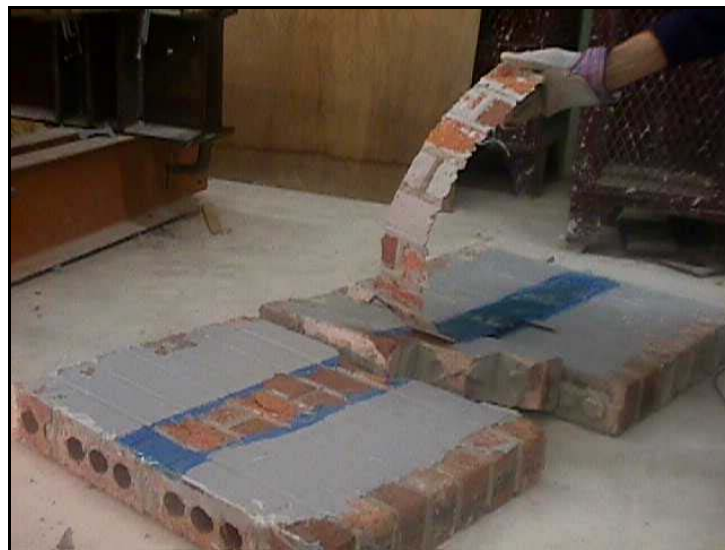
Fig. 2.3.5b*** Debonded laminate after failure
