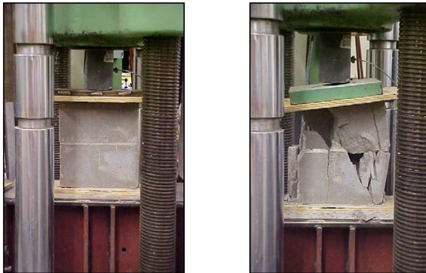
Fig. A.1.2b-c Compression test: prism before (left) and after (right) failure
