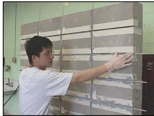
(4) Installation of FRP rods
