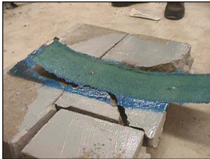
Fig. 2.3.5d* Edge of the specimen after debonding failure
