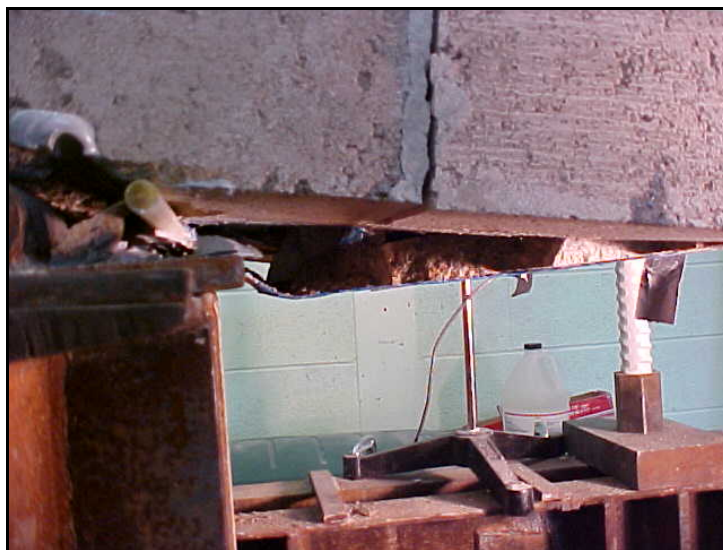
Fig. 2.3.5j Pull-out of NSM rod from the groove
