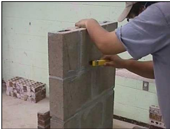
Fig. 2.3.3a Cleaning of the wallettes with a steel brush
