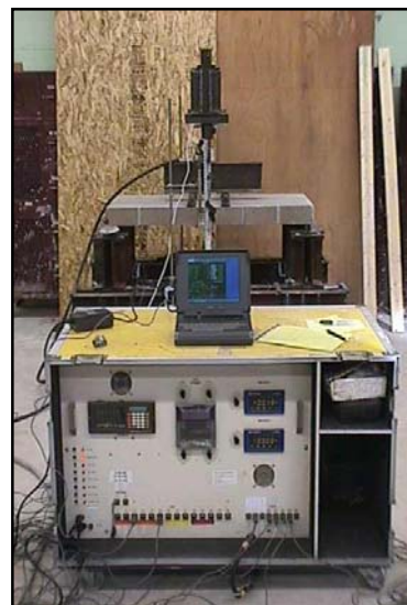
Fig. 2.3.4.2b Data Acquisition System
